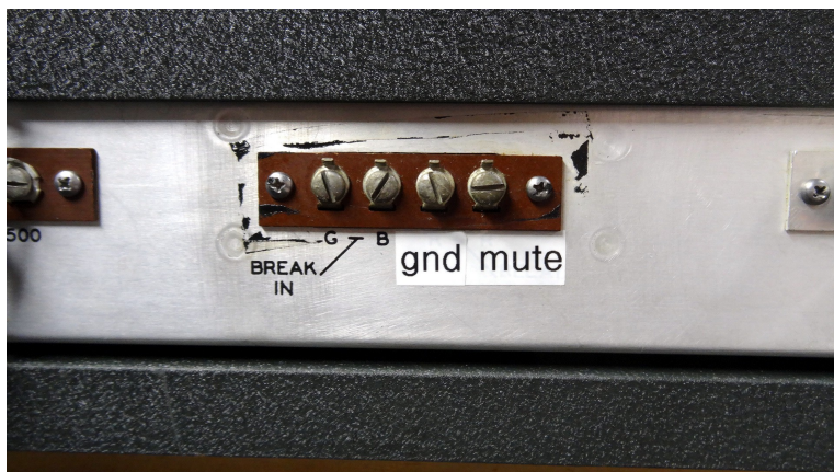
The 75A1 rear panel terminal strip. Relabeled previous relay terminals 3 and 4 to ground and mute. Mute to ground mutes the receiver.
